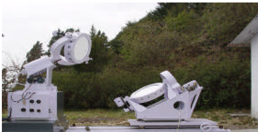
Figure 1. The 45-cm coelostat for the 25-cm, f/66 off-axis Skew Cassegrain telescope at ARIES.
